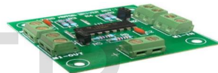
Fig 6. Circuit Board of L293D Motor Driver
